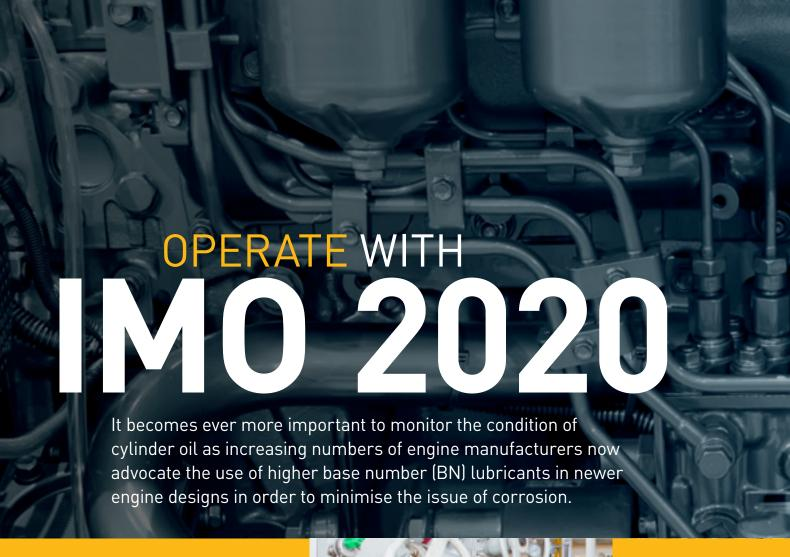
The scrape down oil is continually exposed to acidic combustion products that need to be neutralised before they corrode engine parts. Frequently testing the residual base number of used cylinder lubricant will prevent damage to engine parts by ensuring that alkaline reserve levels required to neutralise the acid are sufficient, preventing unnecessary corrosive damage to costly engine components such as cylinder liners.
